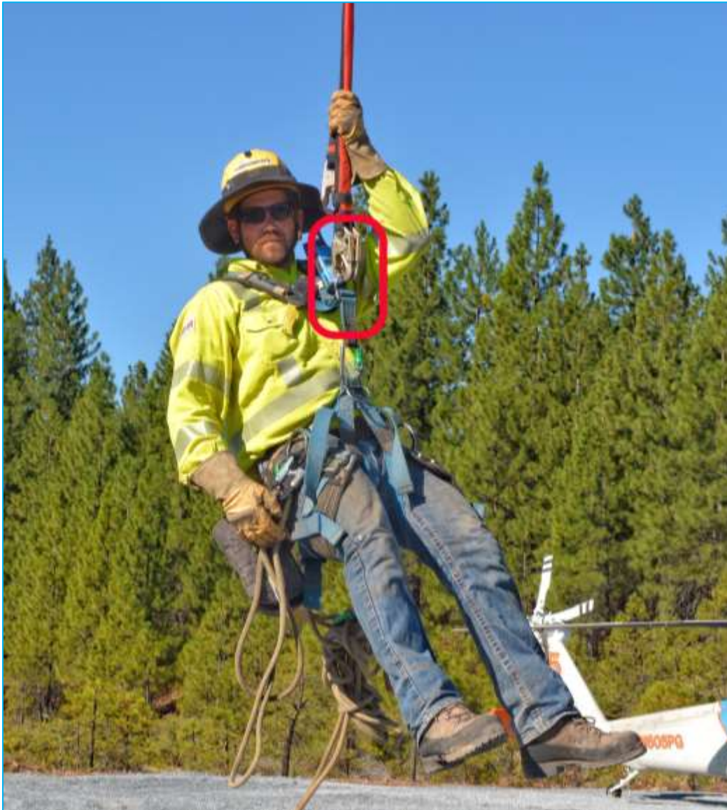
Figure 10: HEC Employee Suspended Using the Front Sternal D-Ring
