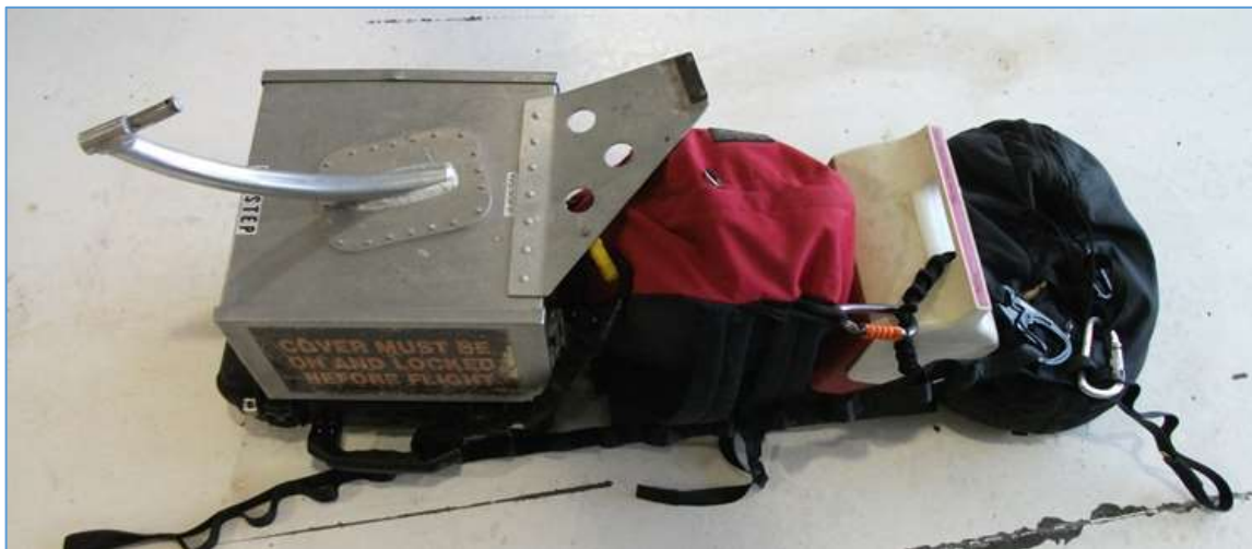
Figure 16: Daisy Chain Securing Cargo
