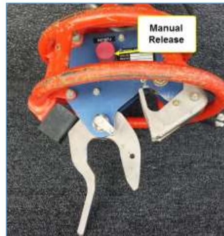
Figure 21: Keeperless Remote Hook – Open Load Beam
