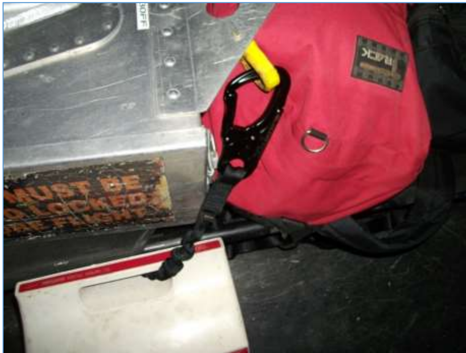
Figure 17: Carabineer Strap Used to Secure Cargo to Daisy Chain
